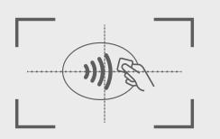
The symbol must be placed exactly over the center or strongest point of the contactless antenna "read area" of the terminal. In some instances, this may require the Contactless Symbol and the payment brands be separately displayed on the reader.
