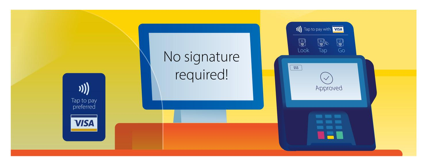
When customers tap to pay with their contactless chip card or payment-enabled mobile or wearable device at a contactless-enabled terminal, the card or device communicates via an NFC antenna and creates a one-time code that keeps the transaction secure. In addition, customers can't pay accidentally. Their card or device must be within 2 inches of the contactless-enabled terminal for a transaction to occur, and the checkout terminal will only read one payment method at a time.
