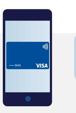
In addition to contactless chip cards, contactless payments can be made through payment-enabled devices, including mobile phones (e.g. Apple Pay, Google Pay) and payment-enabled watches. Payment-enabled devices rely on the same secure NFC technology provided by contactless chip cards, except that they access credit or debit card information that is stored securely in a wallet app on the device.
